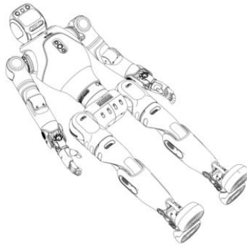
Step3: Switch to Zero-Torque Mode After the Robot is Fully Flat
